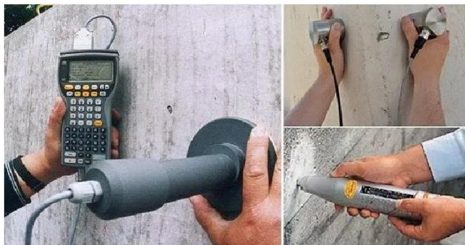
Gambar B.1.9. Pengukuran/pengujian kekuatan beton Sumber: https://theconstructor.org/practical-guide/non-destructive-testing-of-concrete/5553/
