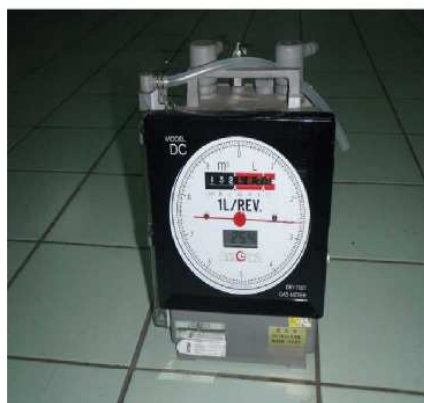
Dry Gas Meter
