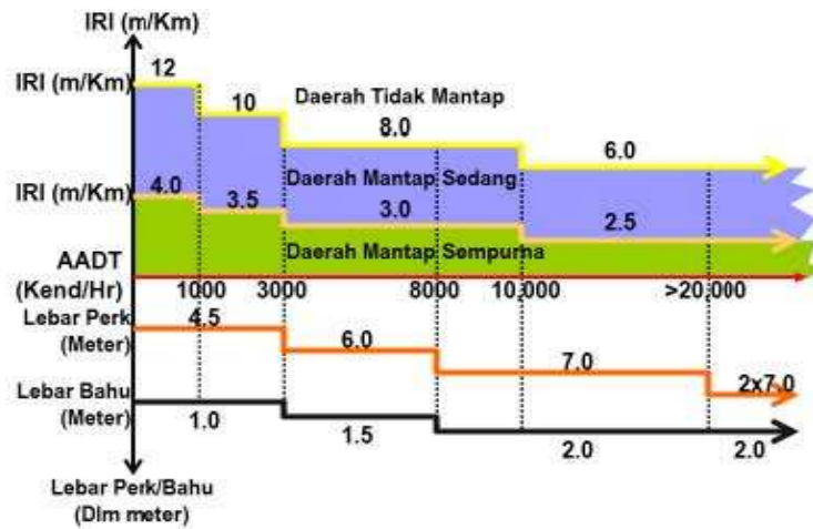
Penanganan Segmen Jalan Berdasarkan Kelayakan Ekonomi Berdasarkan Mid Life AADT (Classification of Treatment Type and Code Ex-IRMS)
